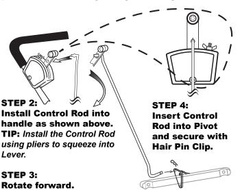
Assembly is complete. Set the stop on the Control Assembly for the desired setting and your spreader is ready to operate.
